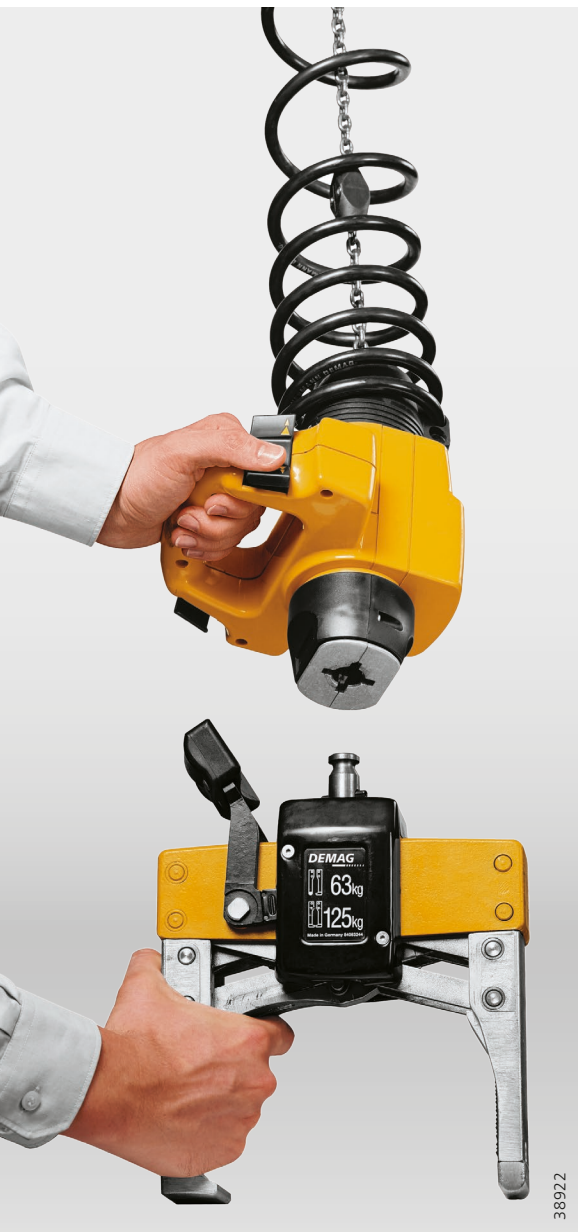
Quick-release coupling as an interface
