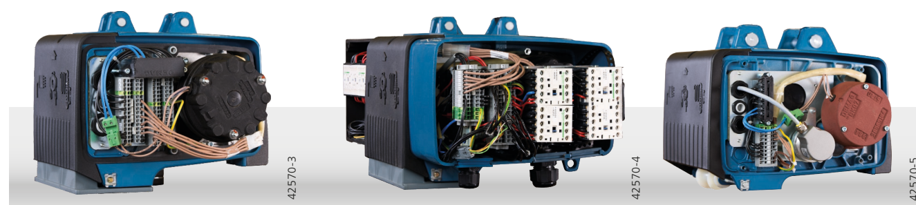
Variable control with customer-specific inverter (DC-ProFC)
