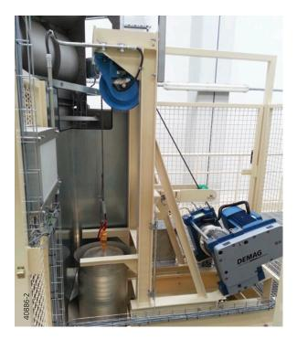
GDR basic hoist: stationary unit as an installation component
