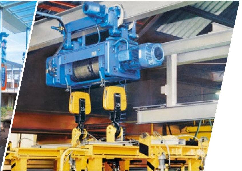
DH hoist unit with two hook lead-offs for transporting mould jigs without any hook travel
