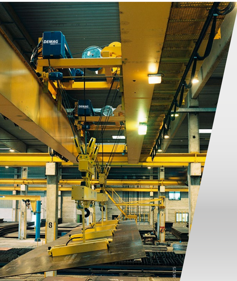
Coaxially coupled hoist unit with angular gearbox, type GW
