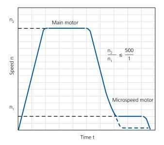
By selecting the motor and gear unit, the speed ratio can be set over a wide range.
