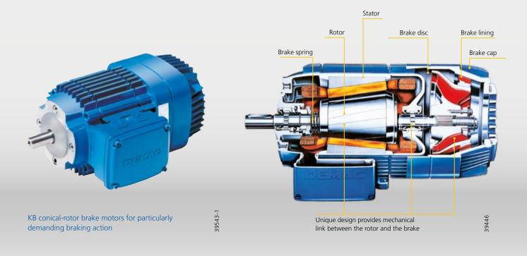
Demag KB conical-rotor brake motors with outputs up to 55 kW and a cyclic duration factor of 40% operate on a unique braking principle:
