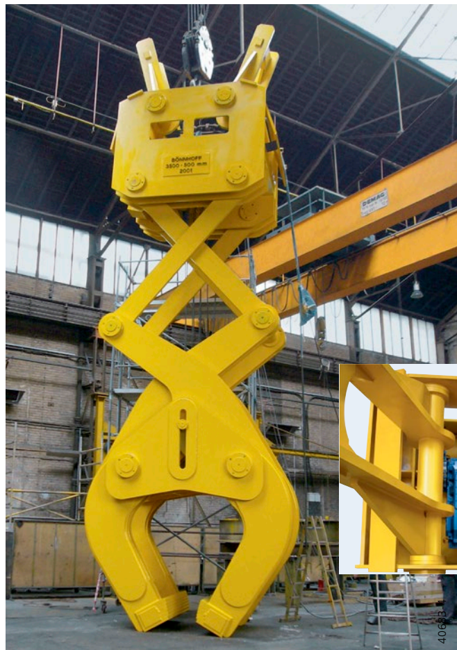
MPW open winch unit employed in a gripper system for transporting steel slabs
