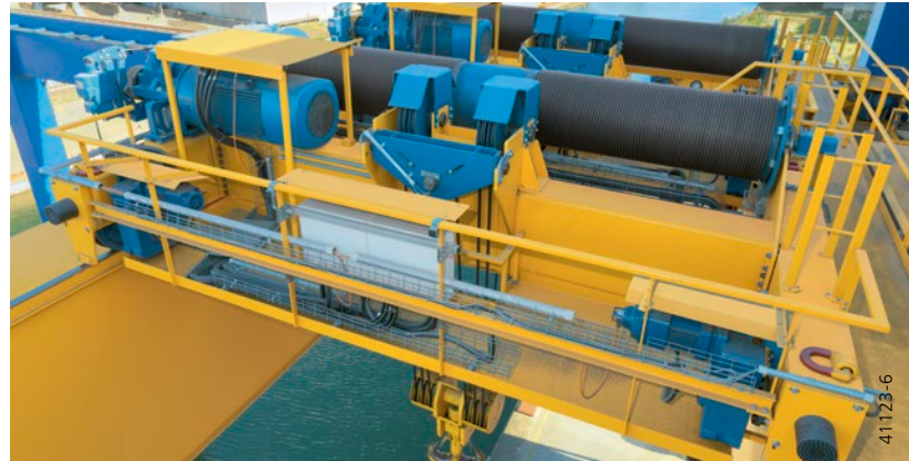
Two 125-tonne MPW crabs for quayside handling with weather-protection equipment for operation outdoors
