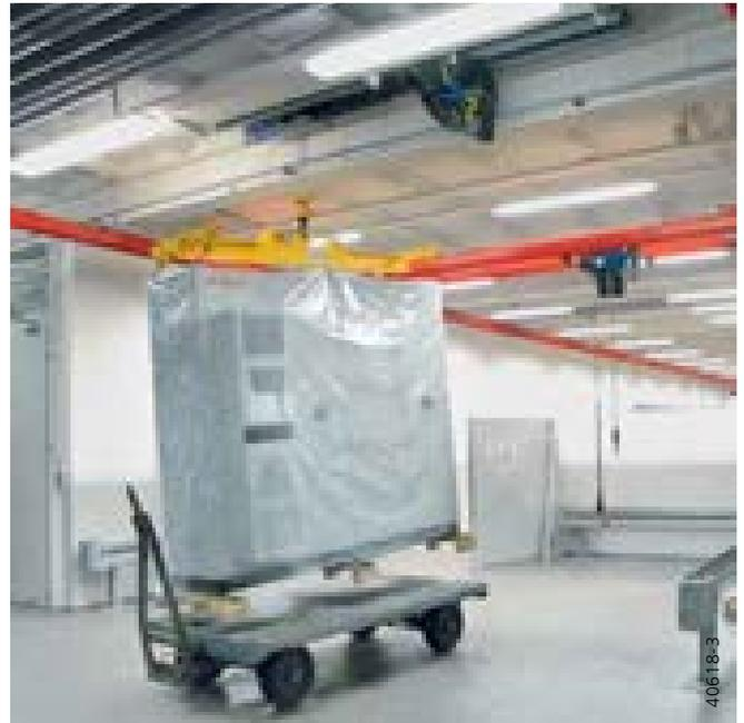
KLDC low-headroom travelling hoist with extended hook lead-off (for big bags)
