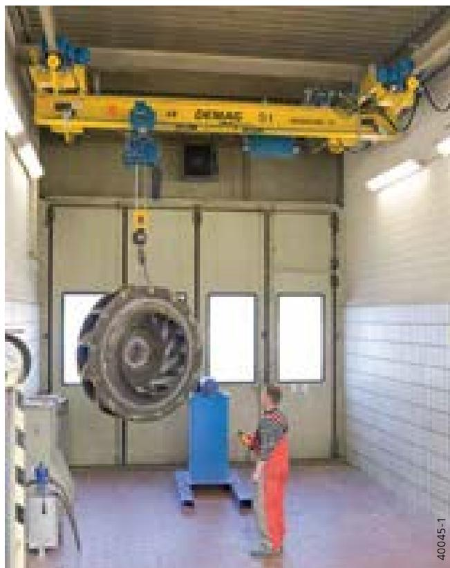
Minimum travelling chain hoist approach dimensions thanks to suspension crane end carriage based on DC chain hoist trolleys
