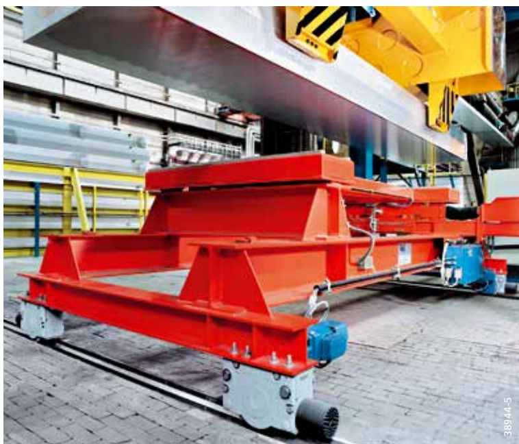
Four-wheel trolley controlled by a frequency inverter for smoothly moving blocks of aluminium
