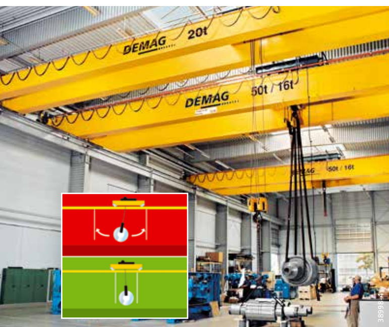
Crane loads can be positioned quickly and accurately, since load sway is virtually eliminated
