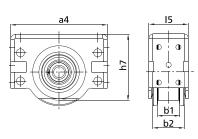
(RS with spheroidal-graphite cast-iron travel wheel with two flanges)
