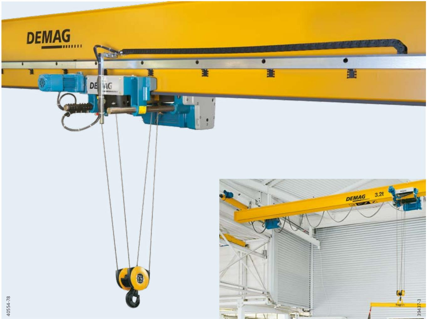
Compared to conventional trailing-cable systems (see small photo), energy chain systems offer improved clearance dimensions. This provides additional safety if the crane has to travel over high workshop equipment or parts of machinery, for example.
