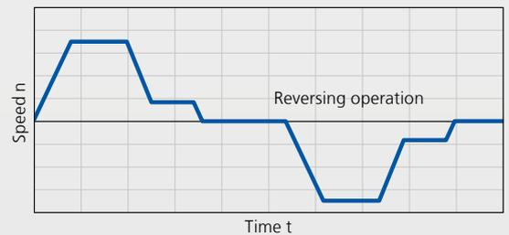
With their integrated flywheel mass, ZBF motors ensure particularly gentle acceleration and deceleration, while the KBF motor additionally accommodates extremely high braking energy.
