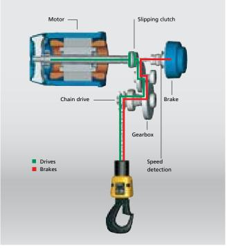
Improved safety: brake/slipping clutch system
