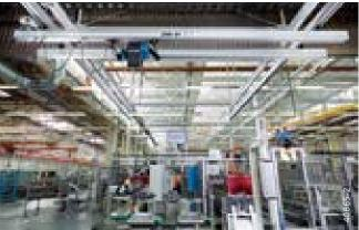
Ergonomic operating sequences can be implemented thanks to the very good trolley running characteristics and the low deadweight of the installations. Reduced loads result in lower absenteeism due to illness and greater employee satisfaction.
