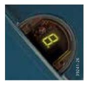
Display for elapsed operating time counter and operating statuses
