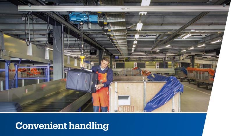
The Demag SpeedHoist is specially designed for fast load handling applications with loads weighing up to 80 kg or 160 kg. The D-Grip control handle enables the load to be guided particularly easily and precisely, in exactly the same way as you move your hand.
